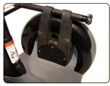
Step 6 Thread three 18mm hex fasteners through the Support and into the threaded inserts in the Gearbox. Once all three fasteners are installed, tighten using a 4mm hex wrench. Torque to 8.0 N-m
