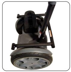
Step 4 Thread three 18mm hex fasteners through the Support and into the threaded inserts in the Gearbox. Once all three fasteners are installed, tighten using a 4mm hex wrench. Torque to 8.0 N-m.
