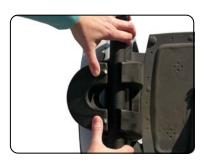
**Step 8** Thread two 35mm hex fasteners with washers through the holes in the Cap and Frame, into the threaded brass inserts in the Support. Tighten with a 5mm hex wrench. Torque to 7.5 N-m.
