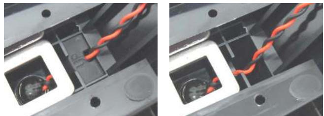
Figure 56: Wire guide present (left) and removed (right)
