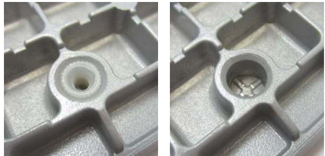
Figure 12: Threaded insert, present (left) and absent (right)
