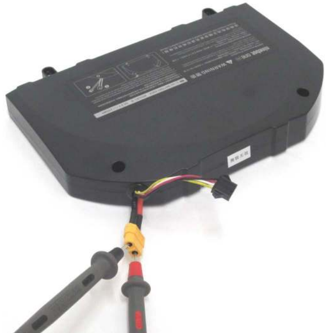
Figure 7: Measure the DC voltage
