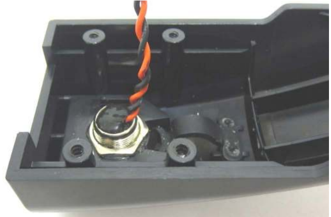
Figure 66: Remove the nut
