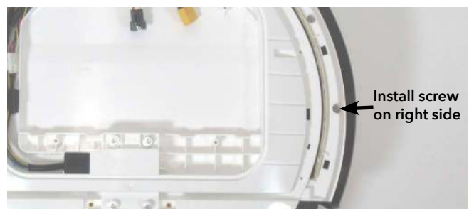
Figure 38: Install the last fastener on the right side panel
