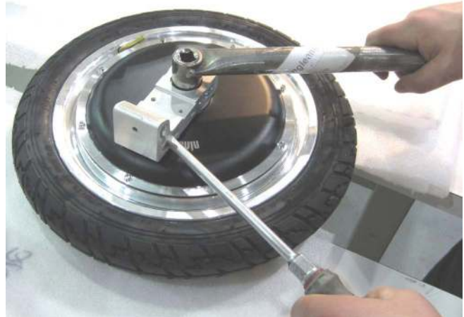
Figure 74: Removing the hub nut
