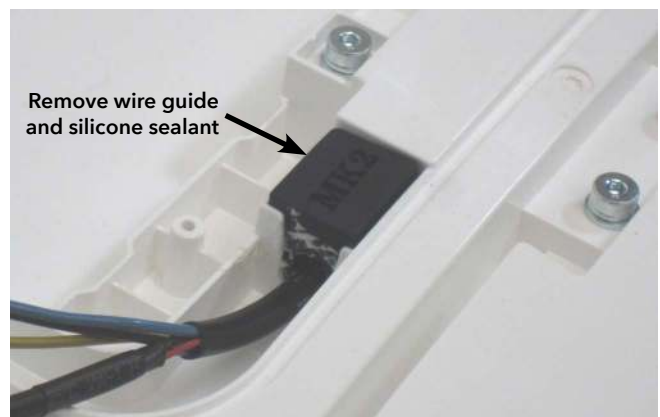
Figure 25: Remove wire guide and silicone sealant
