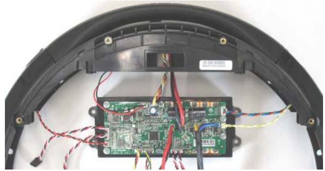
Figure 42: Plug in all wire harnesses
