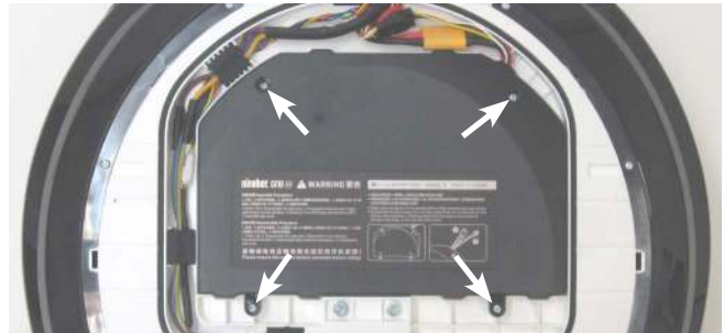
Figure 5: Remove the four screws
