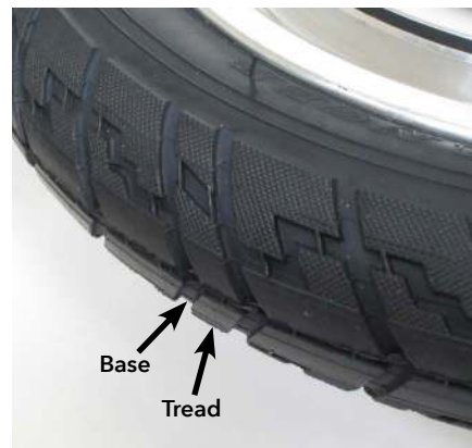
Figure 73: Measuring tread depth
