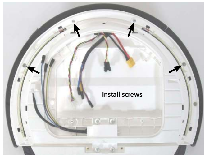
Figure 33: Install four screws
