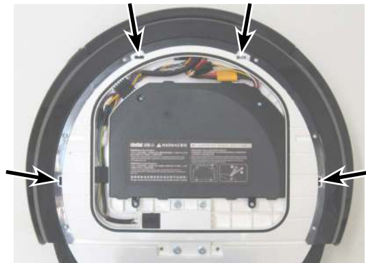
Figure 4: Line up cover tabs with slots in the housing
