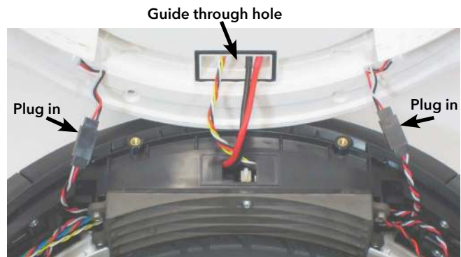
Figure 36: Connect the left side panel to the frame
