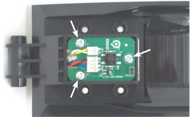
Figure 64: Remove the three screws
