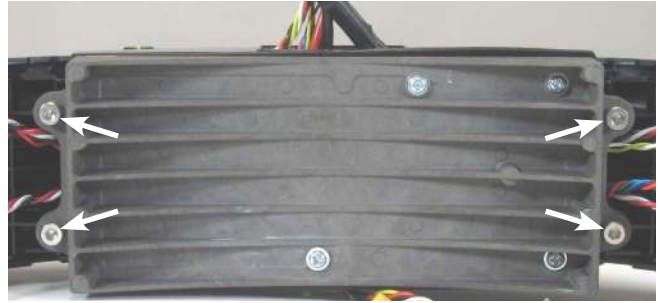
Figure 39: Remove the four fasteners
