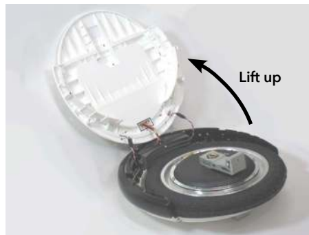
Figure 21: Lift the side panel from the bottom
