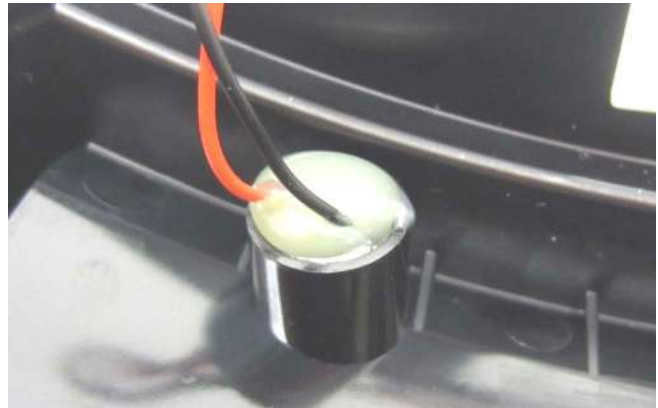
Figure 71: Glue holds buzzer in place
