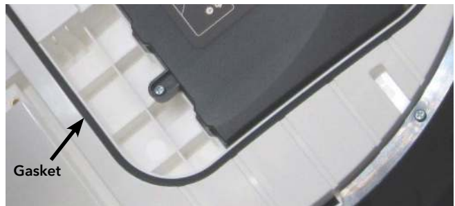
Figure 3: Verify gasket is installed
