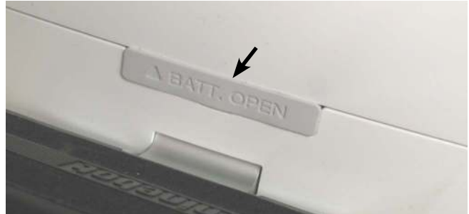
Figure 1: Remove the silicone plug
