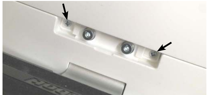
Figure 2: Remove the two Phillips-head screws
