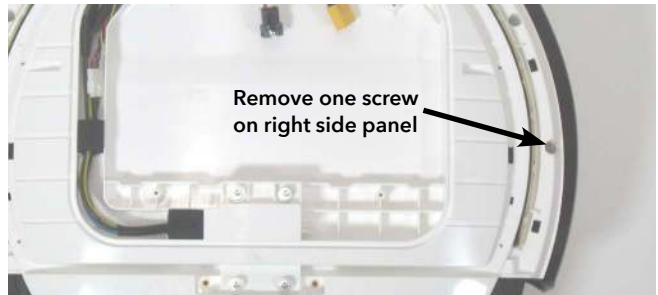
Figure 20: Install the last fastener on the right side panel
