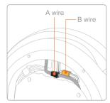
Unplug the black wire (A) first, Pull the connector firmly. Do not pull on the wire itself or you may damage it.
