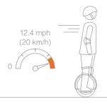
Do not accelerate when the One S1 tilts back or sounds an alarm. Do not attempt to override the speed limiter.
