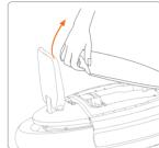
Power off the vehicle and Use a Phillips-head screwdriver disconnect the charger. Then to remove the two screws. Then, then unplug the yellow wire (B). remove the rubber plug on the with a firm tug, use your hand to lift and remove the battery cover.
