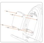
remove the four battery screws as the battery cover to snap it in to install the battery cover shown.
