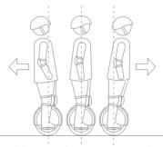
5 Place both feet on the pedals and practice traveling forward and backward by controlling your body's center of gravity.
